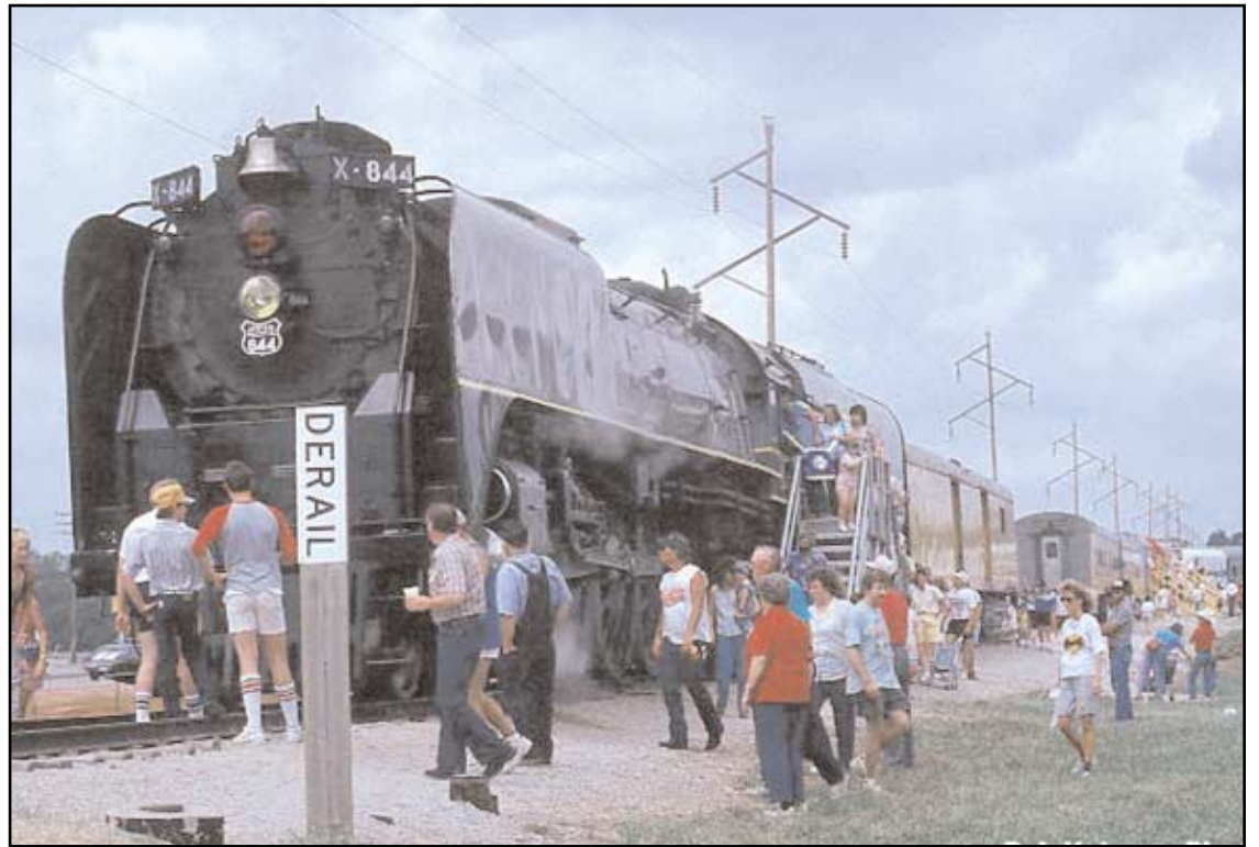
The last steam locomotive built for Union Pacific, delivered in 1944, was Northern No. 844 (above). The Northern-class steam locomotives, with a wheel arrangement of 4-8-4 and capable of speeds exceeding 100 mph, were used by most large U.S. railroads in dual passenger and freight service.
