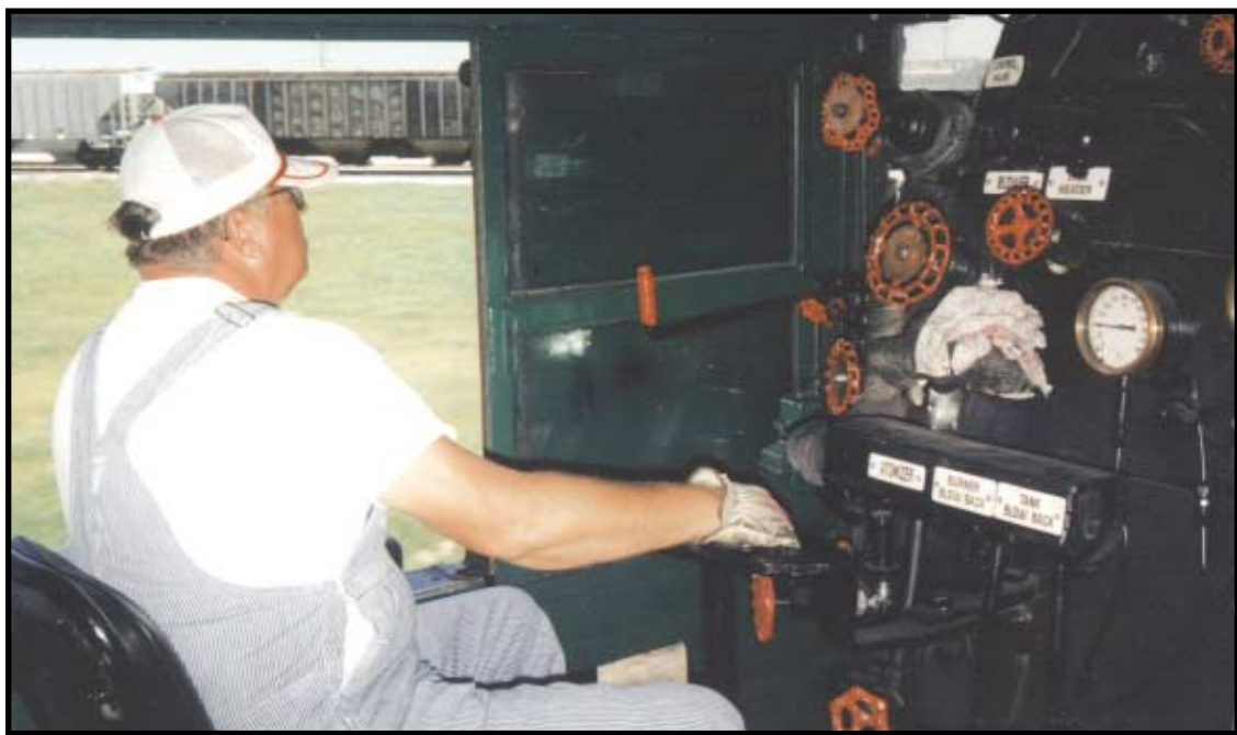
Lynn Nystrom, serving as fireman aboard Challenger #3985, keeps an eye on the gauges and adjusts the valves. Although he worked previously as an engineer, Nystrom wears many hats to keep the steam excursions running. "The key is to always watch the water pressure," Nystrom cautioned.
