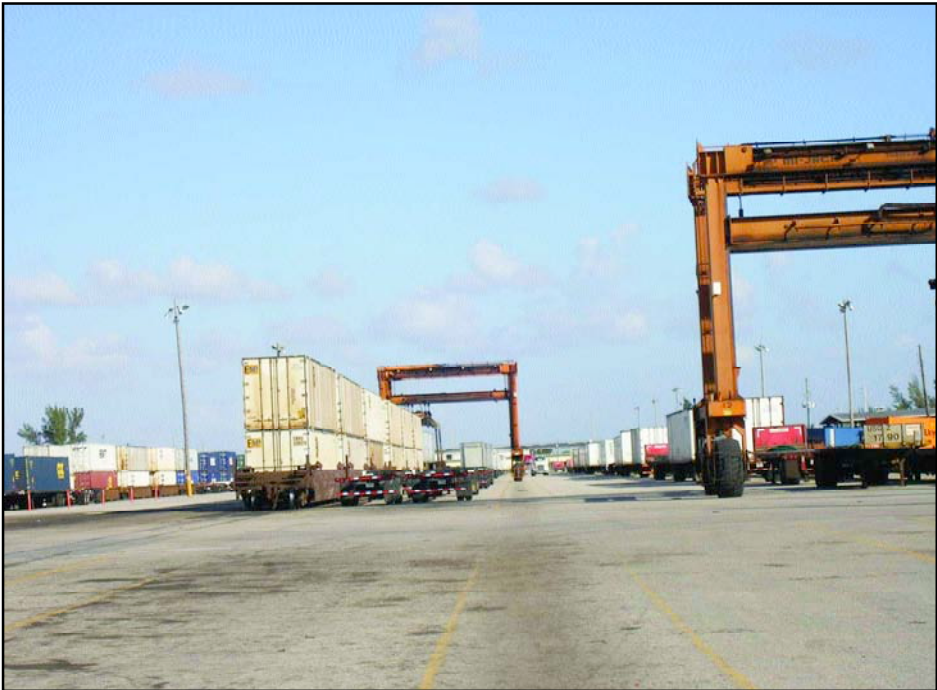
Note the two rubber-wheeled cranes that lift the containers to and from double-stack rail flatcars in the Miami FEC yard. Similar operations occur at PARSEC-operated facilities in Jacksonville and Ft. Lauderdale, where the UTU also represents ground-service employees.
