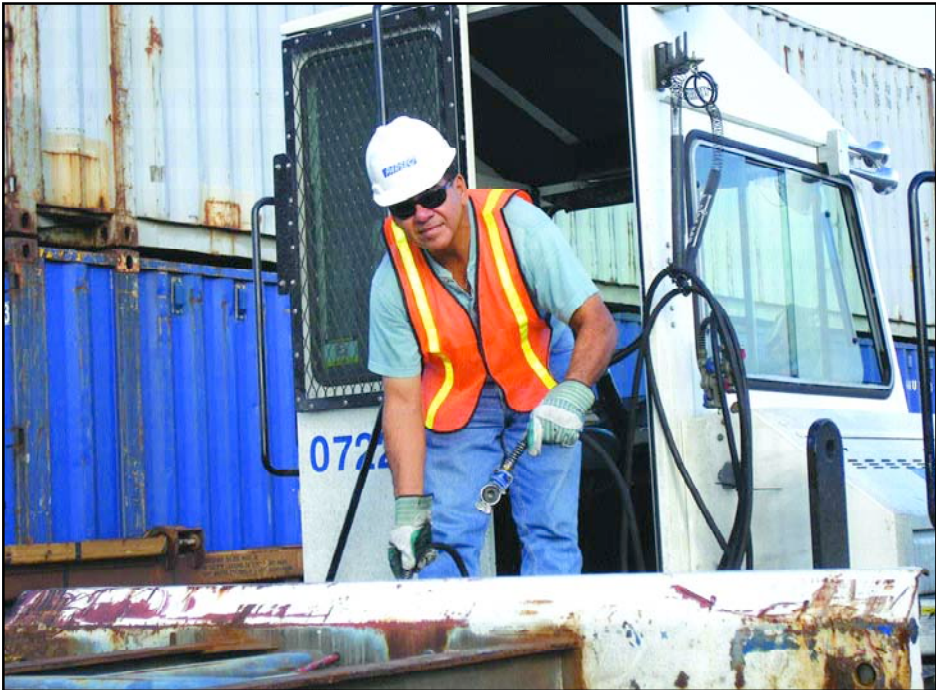
At the FEC intermodal terminal in Miami, arriving cargo containers are removed by cranes from intermodal flatcars and positioned aboard a wheeled chassis for subsequent pick up by local truckers. Connecting air-brake hoses to a chassis at the FEC Miami terminal is Juan Ucanan, president of Local 1900, Miami, Fla.
