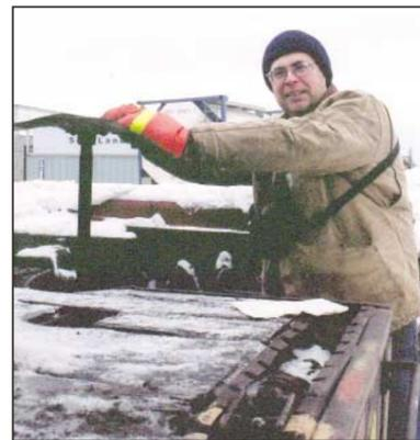
Conductor John Fleming sets the hand brakes on a container car. Most consumer goods arriving in Alaska are containerized. The railroad also hauls much heavy equipment north for oil exploration, earthmoving and pipelines.
