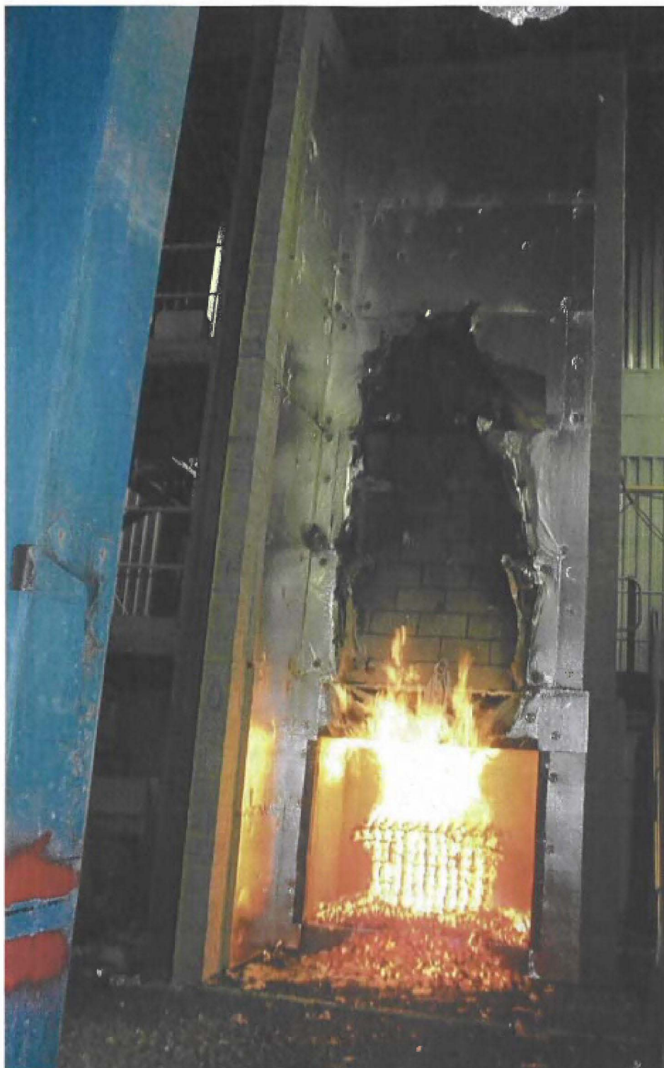
47. KINGSPAN BS 8414-1 Old Technology Phenolic Test 2005 – 25minutes in
