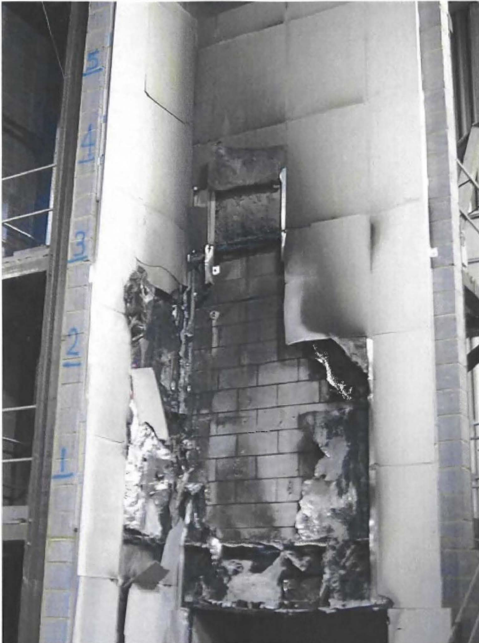
48. Old Technology Phenolic with non combustible board cladding – BS 8414-1 2005
