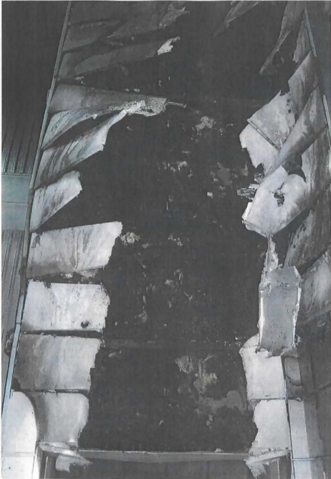
46. Sotech Rainscreen BS 8414-2 test with New Technology K15 MSK December 07
